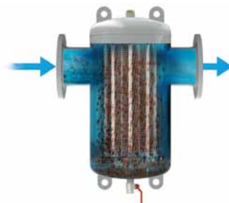
Exdirt Function Diagram
